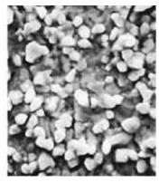
**LEFT**: ORMECON CSN Classic highly crystalline tin layer lowers copper diffusion speed. **RIGHT**: Tin deposit using competitive process reduces shelf life and performance.
